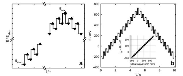
**Figure 5.** (a) Squarewave voltage waveform. Down-pointing and up-pointing triangles marks where the reverse and forward current is sampled, respectively. (b) Simulated waveform (gray) and waveform from sensor platform (black) obtained by multiplying the squarewave current  $I_R$  with the load resistance,  $R$ . The inset shows the relationship between actual and simulated waveforms.
