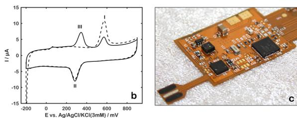
**Figure 1.** (a) detection of glucose (b) platform can do other electrochemical techniques(---) and second (—) scan. (c) Electrochemical sensor platform, dimensions of body: 29 × 21 × 1.2 mm, weight: 1.2 g.
