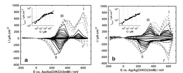
**Figure 6.** Baseline corrected coarse cyclic squarewave voltammograms (second scan) from (a) commercially sourced electrodes and potentiostat, and (b) sensor platform with integrated electrodes and electronics. The dotted lines (---) represent the signals which satisfies  $I \geq I_{III}$ . The insets show the corresponding calibration curves from Eq. (1).
