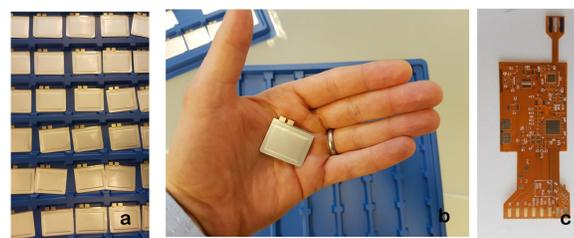
**Figure 3.** (a) The thin lithium polymer battery (b) The thin lithium polymer battery (c) The biosensor and electronics are mounted on the same flex pcb.
