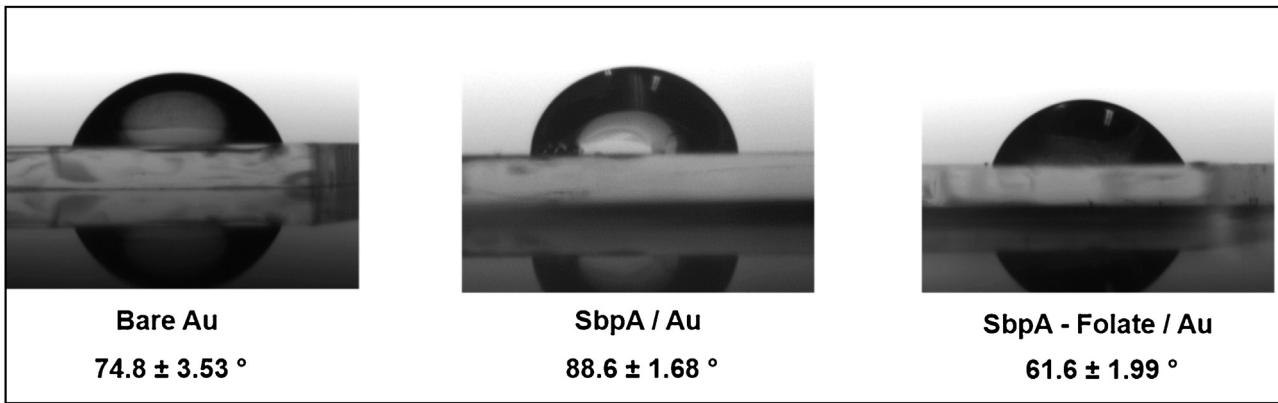
**Fig. 1.** Water contact angles for bare gold, S-layer protein (SbpA) and functionalized SbpA-folate layers.
