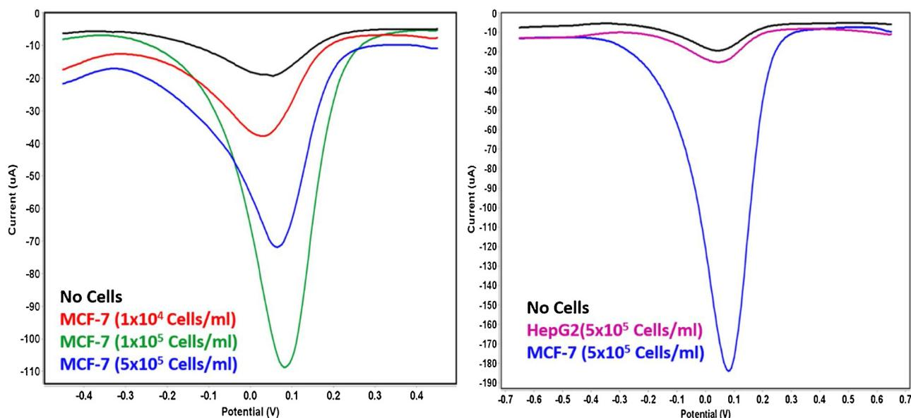
**Fig. 5.** (a) Square wave voltammograms for MCF-7 breast cancer cells captured on the modified SbpA-folate/Au electrode at different concentrations and (b) Square wave voltammograms for detection of MCF-7 and HepG2 cancer cells at concentration  $5 \times 10^5$  cells/ml.
