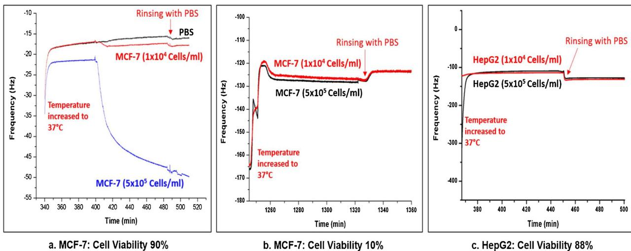
**Fig. 3.** Frequency shifts recorded at the 5th overtone as function of time for the capturing of cancer cells by the functionalized SbpA-folate/Au QCM-D-sensor at two different concentrations ( $1 \times 10^4$  and  $5 \times 10^5$  cells/ml), (a) capturing of MCF-7 breast cancer cells (cell viability 90%), (b) capturing of MCF-7 breast cancer cells (cell viability 10%), and (c) capturing of HepG2 liver cancer cells (cell viability 88%).
