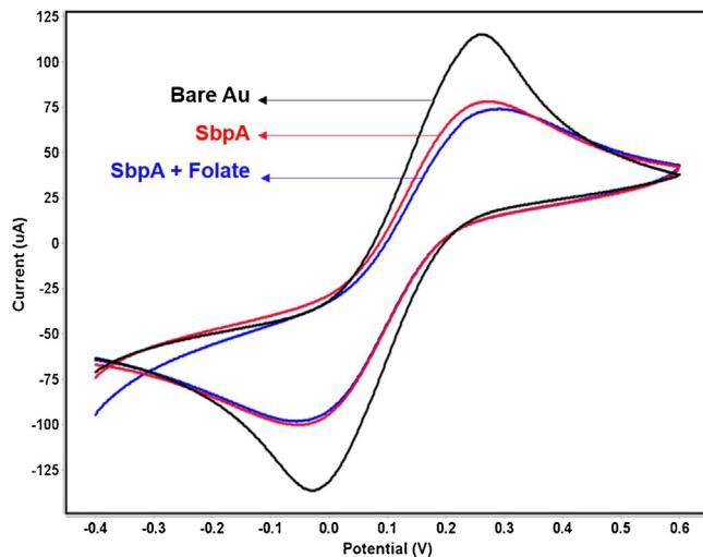
**Fig. 4.** CV spectra of the bare gold electrode and S-lattice with or without folate on gold electrode in  $10\text{mM K}_3[\text{Fe}(\text{CN})_6]$  containing  $100\text{mM KCl}$  at a scan rate of  $50\text{ mV/s}$ .
