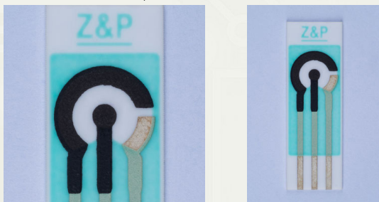
1.2.4.3 Bare Graphene Sensor A-AC-GrGr-110-N
